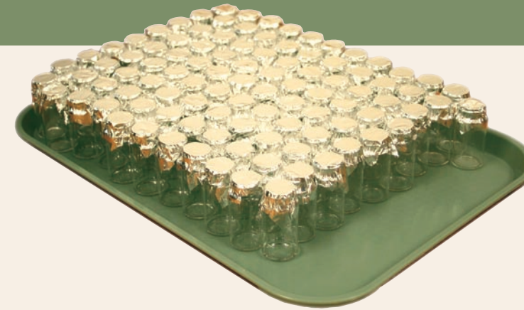
(left) Glass vials are carefully cleaned for sample storage. Plastic is avoided as much as possible to minimize organic matter contamination.
