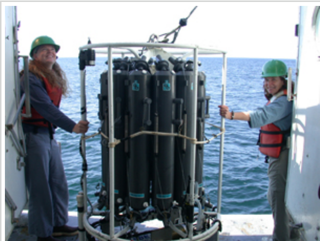
Deploying the Conductivity, Temperature and Depth rosette with water sampling bottles attached.
